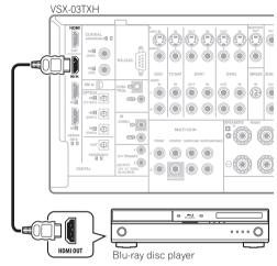
The diagram shows a basic setup of this receiver together with a Blu-ray disc player, with HDMI connections. If your Blu-ray disc player offers multi-channel analog audio outputs, see Using XM Radio on page 56.
